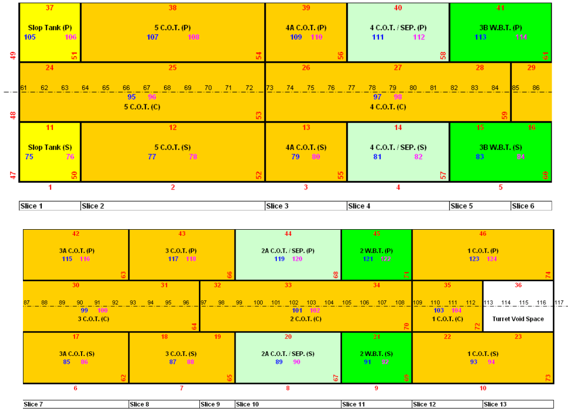
Figure 1: FPSO Layout (cargo region)
